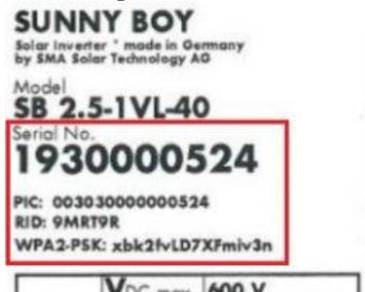
Information such as the serial number, PIC and RID can be found on the inverter label and the documentation that comes with the inverter. After the device is installed, information on the label may become difficult to read. If this information is not on hand (after leaving the installation site), taking a picture of the label and having it readily available will be useful for future reference. This information is necessary for registration to Sunny Portal and may be needed during commissioning.
